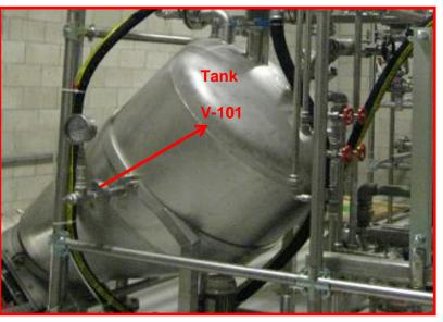
V=22 lt (2 kg of biomass/cycle) Pmax = 26 barTmax=227 °C Pre-heating jacket V=10 lt Temperature and pressure control system
