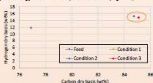
Figure 2: H and C elemental composition on dry basis of feeds and products after hydrotreatment
