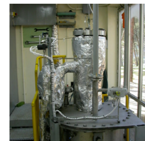
Figure 2. Steam explosion pilot unit of Advanced Biofuels and Bioproducts Unit at CIEMAT.
