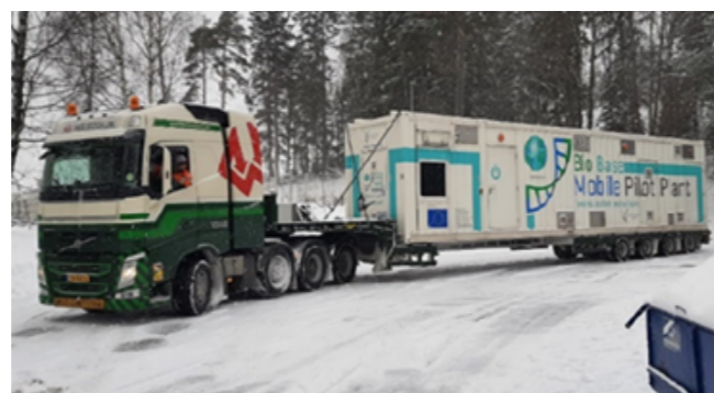
Figure 4. Bio Base Mobile Pilot Plant (BBMPP), a containerized mobile unit dedicated for gas fermentation processes. BBMPP at the site of Arcelor Mittal Ghent (Belgium) in the framework of BIOCON-CO2 project (top picture) and BBMPP loaded onto a truck and delivered to its new location at VTT (Finland) (bottom picture)
