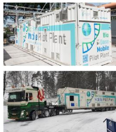
Figure 4. Bio Base Mobile Pilot Plant (BBMPP), a containerized mobile unit dedicated for gas fermentation processes. BBMPP at the site of Avonor Metall Oyj (Bergby) in the framework of BIOCO 2 project (top picture) and BBMPP loaded onto a truck and delivered to its new location at VTT (Finland) (bottom picture)
