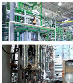
Figure 3. DFB purification pilot and syngas ultra-purification unit at VTT Bioruukki pilot centre
