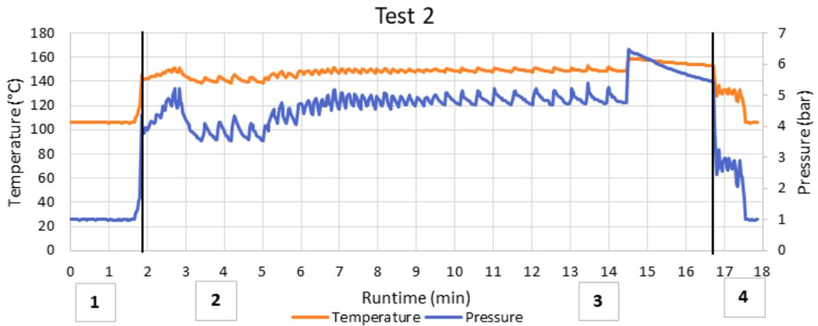
Figure 27: Temperature and pressure trend of steam explosion II
