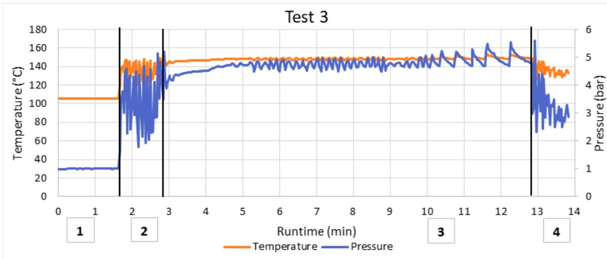
Figure 30: Temperature and pressure trend of steam explosion III
