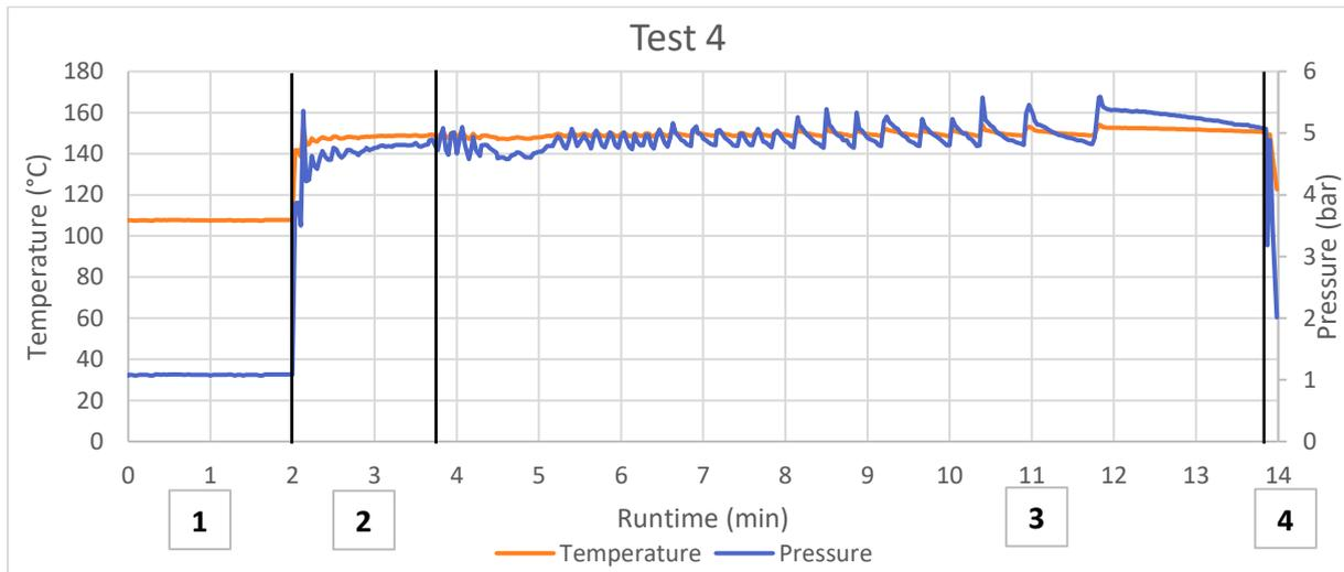
Figure 31: Temperature and pressure trend of steam explosion IV
