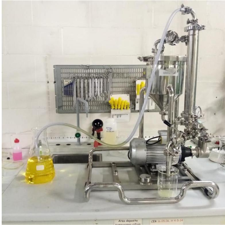
**Figure 25: Membrane small scale plant**
