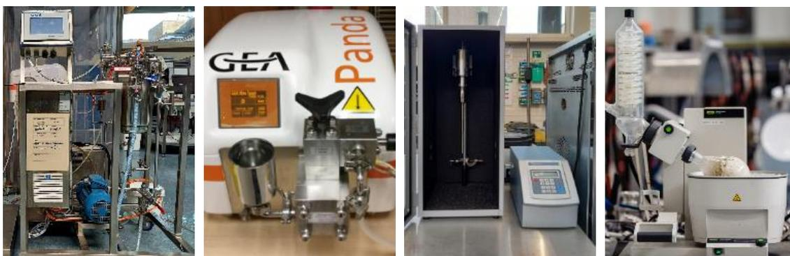
Figure 3: Equipment used for DSP of TAG at BBEP: ceramic filtration unit, high-pressure homogenizer, sonicator, rotavapor (from left to right).
