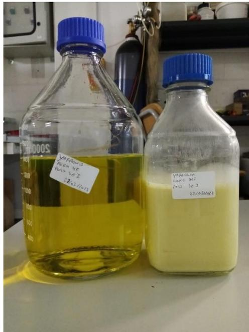
Figure 24: Permeate and concentrate samples after microfiltration steps
