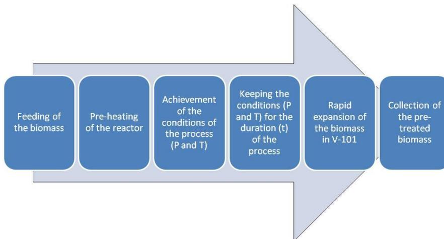
Figure 14: Steam explosion cycle
