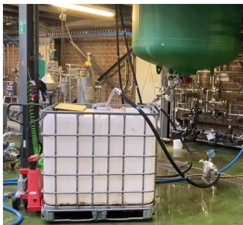
Figure 26: Set-up for separating heavy phase from the light phase.
