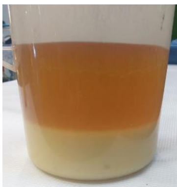
Figure 12: Two phases after solvent extraction
