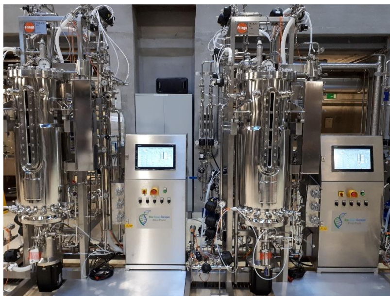
Figure 2: Pilot-scale 150 L fermentation bioreactors for TAG production at BBEPP.
