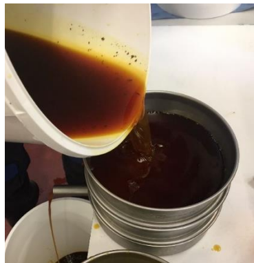
Figure 31: Sieving of the filtrate after chamber filter press.
