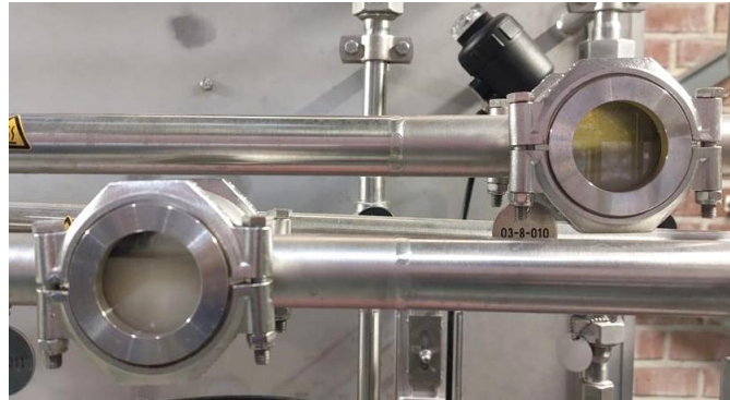
Figure 27: Sight glasses of TSE20 centrifuge with separation of the heavy phase (left) and light phase (right).
