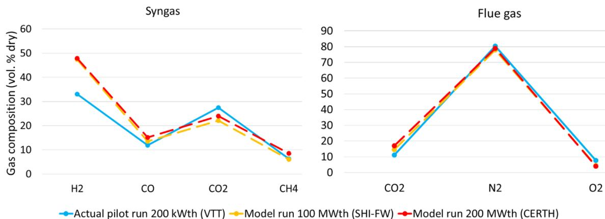
Figure 9. Validation of the 200 MWth DFBG model
