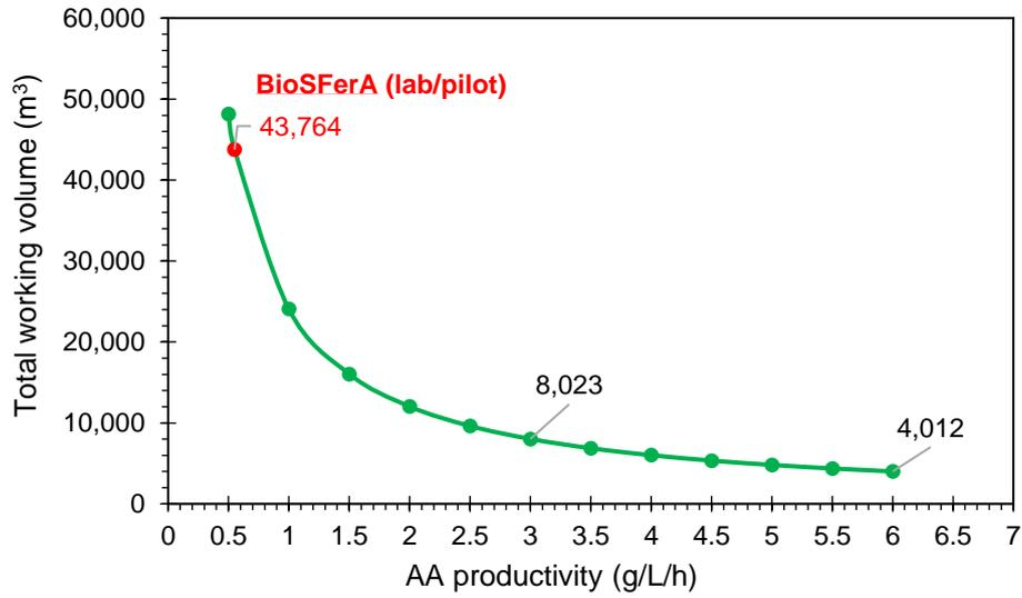
Figure 12. Influence of AA productivity on total working volume (gas fermentation).
