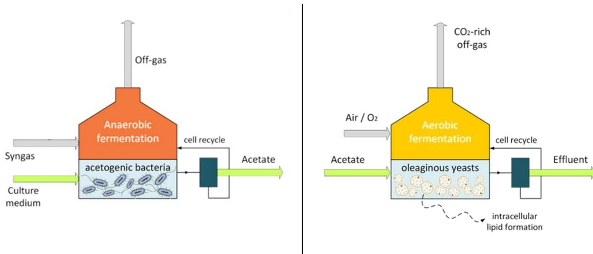
Figure 3. Syngas fermentation (left) and acetate fermentation (right) in a continuous mode [1], [3]
