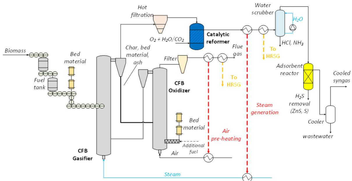
Figure 2. Thermochemical part of the BioSFerA value chain [1], [3]
