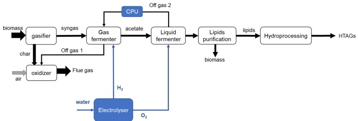
Figure 21. Carbon utilization enhancement through CPU
