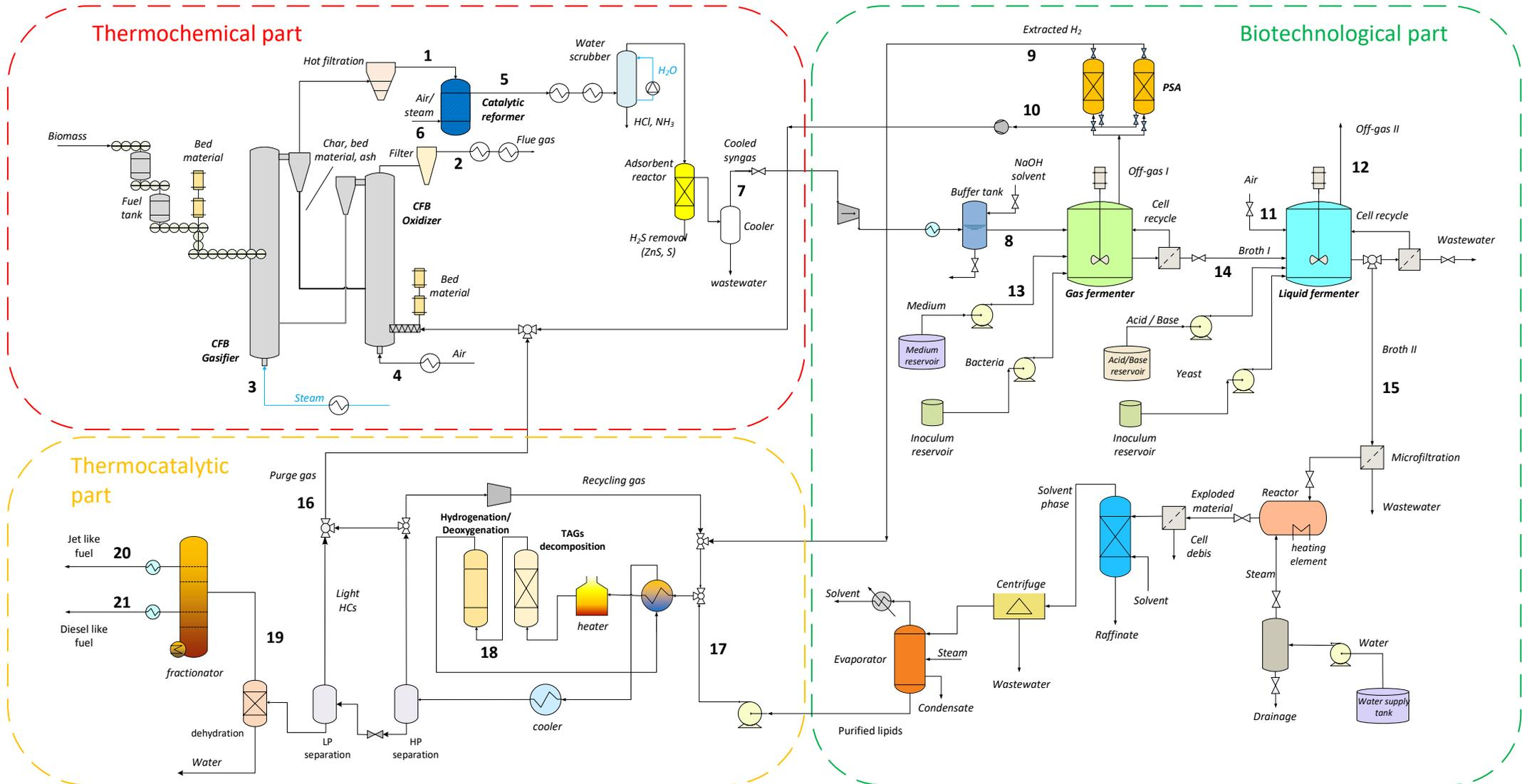
Figure 7. Process Flow Diagram (PFD) for the BioSFeA BtL process chain
