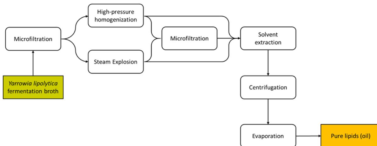
Figure 4. Proposed DSP train for lipids purification [8]
