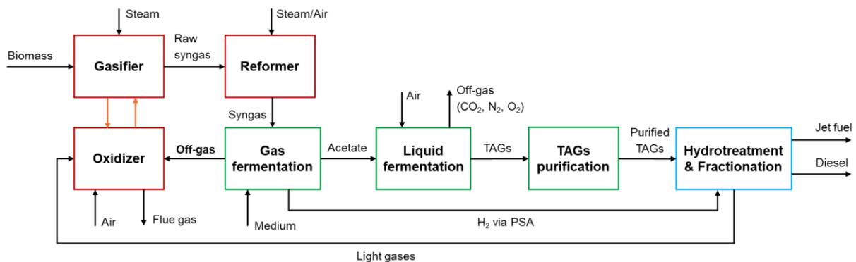
Figure 6. Block Flow of the integrated BioSFerA concept
