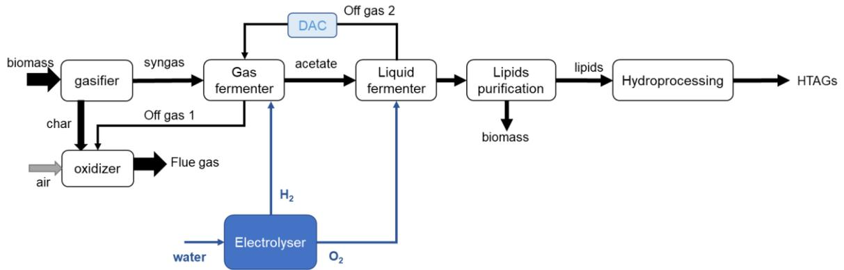
Figure 23. Carbon utilization enhancement through DAC
