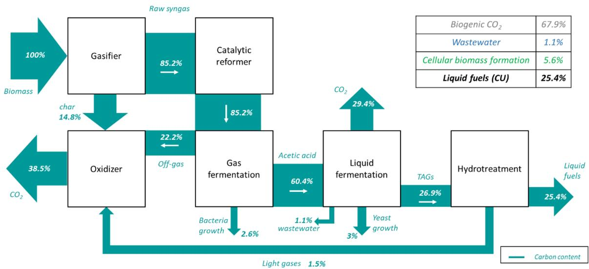
Figure 18. Carbon balance of the integrated concept (BioSFerA 200 MWth full-scale simulations)
