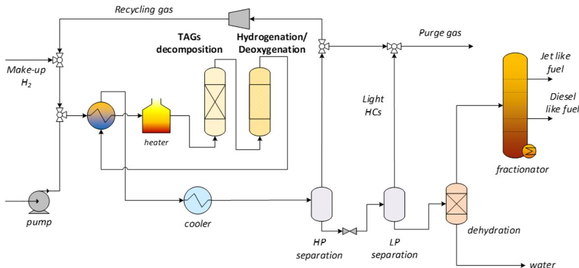
Figure 5. Hydrotreatment of the BioSFerA value chain [1], [3]
