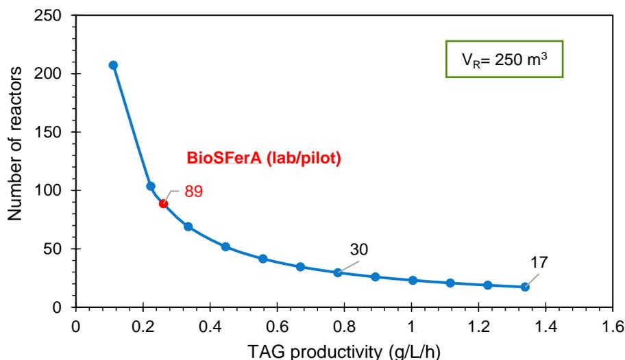
Figure 16. Influence of TAG productivity on total number of reactors (liquid fermentation).
