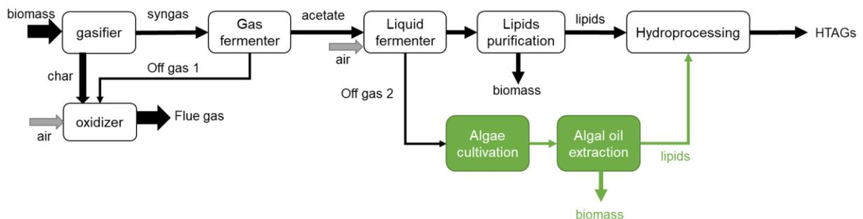
Figure 22. Carbon utilization enhancement through algae cultivation
