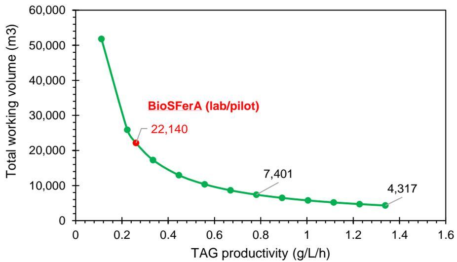
Figure 15. Influence of TAG productivity on total working volume (liquid fermentation).
