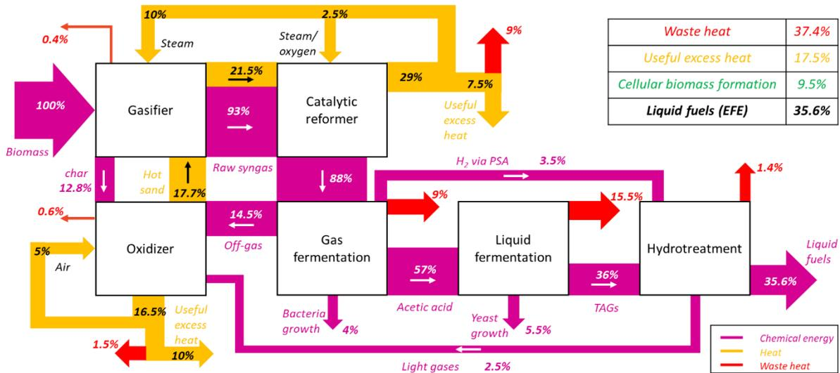
Figure 17. Energy balance of the integrated concept (BioSFerA 200 MWth full-scale simulations)
