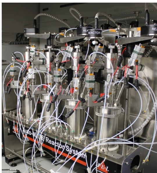
Figure 7: Four parallel 1 L bioreactors for gas fermentation at BBEPP.
