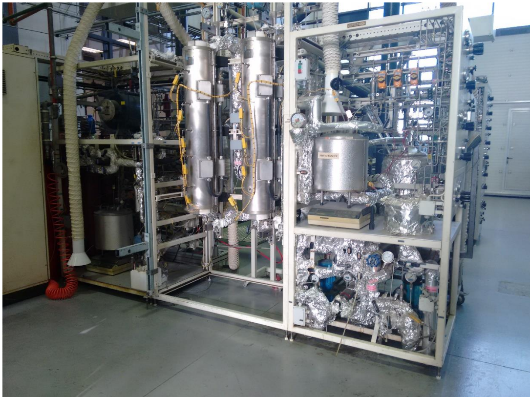
Picture 2 TRL 5 Hydrotreatment pilot plant at CERTH
