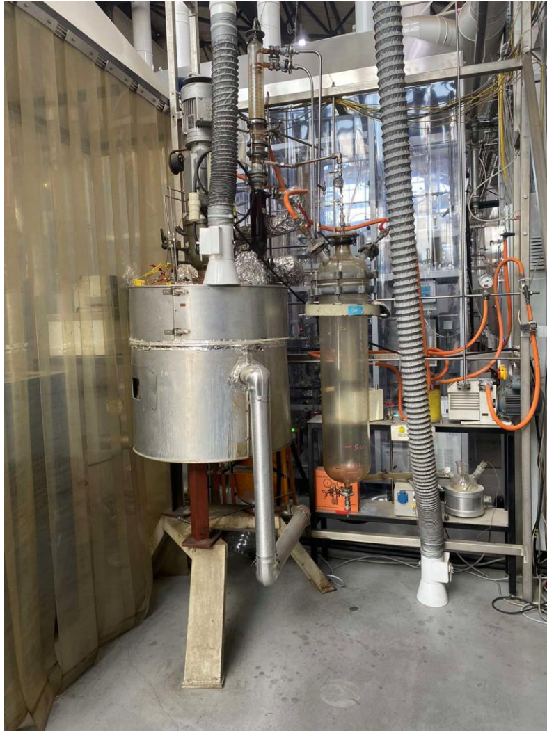
Picture 3 Batch fractionation pilot plan at CERTH
