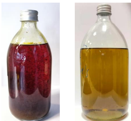
Picture 1 Photos from the real TAGs on the left and from the Model Compound feedstock on the right
